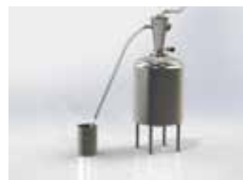
Vacuum Transfer into a Vessel
