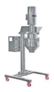
Gansons Multimill is a simple processing solution for sizing of relatively larger solid particles or lumps into comparatively smaller particles with narrow particle size distribution. It has a very small footprint and wide applications.
